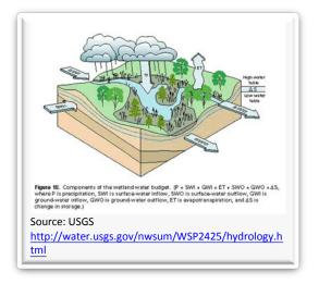
outflows. Water may be stored on the wetland surface, in its soil profile, or both. The accounting of the inflows and outflows with adjustments in storage is the wetland water budget. The presence of water can be described quantitatively using these parameters: probability, frequency, and duration of surface and groundwater. These parameters
