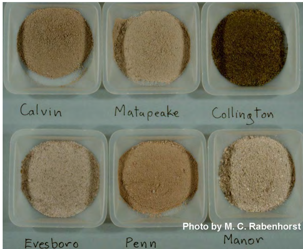
Figure 4-1.—Note the variety in color of uncoated mineral grains, which contribute to the color of soils. Iron oxides were removed from these soil materials, which are from six different soil series that formed in a variety of parent material.
