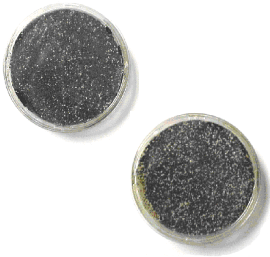
Figure 7-3.—On the left, 70 percent of sand grains coated or masked by organic compounds; on the right, 50 percent of sand grains coated or masked by organic compounds. Photos courtesy of Michael Vepraskas, North Carolina State University.
