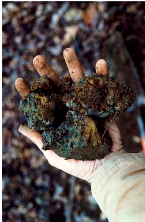
Figure 10-16.—A soil sample taken from the surface horizon of a glauconitic soil. The soil meets the color criteria of NRCS Field Indicator F6 (Redox Dark Surface) because of the dark greenish black color of the glauconite combined with the redox concentrations.
