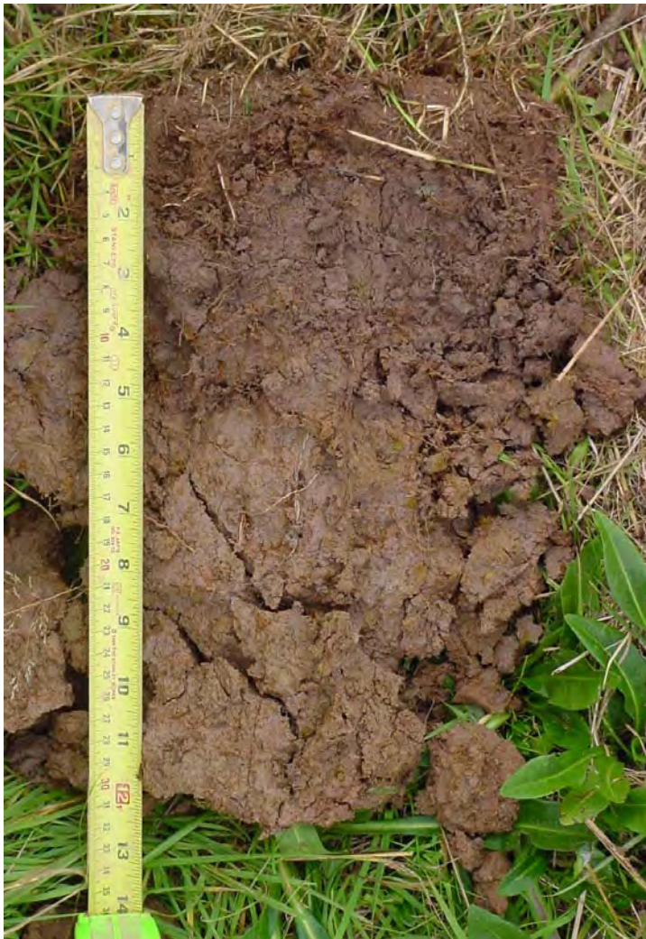
Figure 10-2.—A hydric soil formed in alluvium derived from red parent material. This soil is in a drainage swale at a Mid-Atlantic Hydric Soils Committee study site. The red parent material was confirmed by CCPI testing. The profile is sufficiently wet for a very long period of time and meets Field Indicator F3 (Depleted Matrix).
