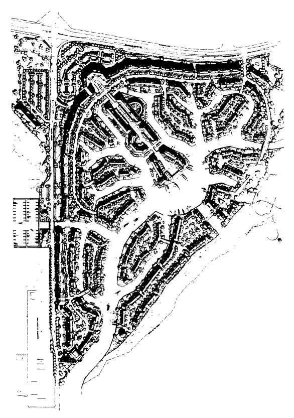
Figure 6. General plan for the Port Liberte waterfront community. The artificial canal system is open to tidal flow on the north, south, and at the main boat entrance at the southeast. The canals shallow from the central trunk to the laterals. Deadends have been virtually eliminated.
