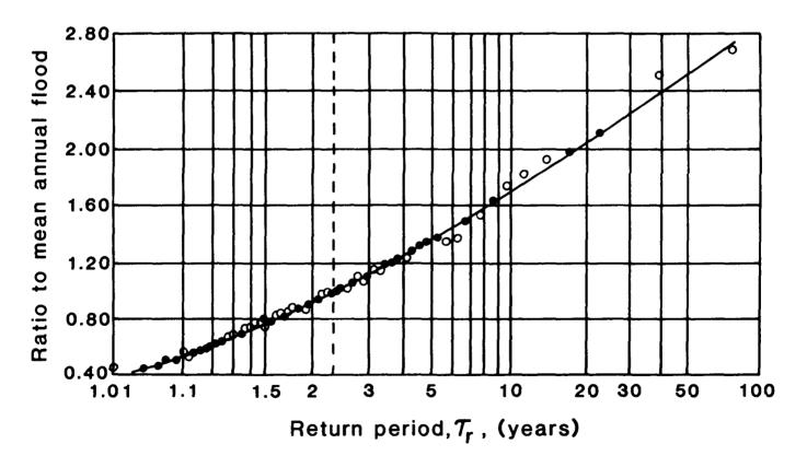
Figure 4. Regional-flood-frequency curve for selected stations in the Youghiogheny and Kiskiminetas River basins (Pennsylvania and Maryland), showing the return time for pulsed events expressed as a ratio to mean annual flood. A reduction in the hydrologic detention of wetlands raises the slope of this curve (U.S. Geological Survey, from Linsley et al. 1975).
