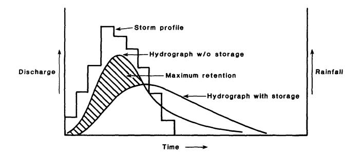
Figure 2. Flood hydrographs for watersheds with and without wetland storage capacity (from Reppert et al. 1979).
