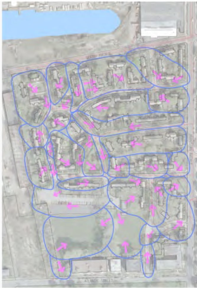
SUB-BASINS & SURFACE WATER FLOW 4.05.2010
