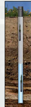
Monitoring Well and Dataloggers
